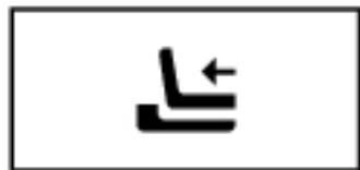
Use this connector to attach the optional docking device, also called an advanced port replicator (APR). A docking device, or APR, allows you to easily use external devices with your computer, such as an external keyboard, mouse, or monitor.
