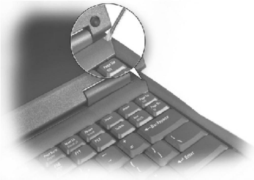
5. To release the keyboard from the palm rest, use a small, flat-blade screwdriver or plastic scribe to pull up on the scalloped edge of the blank key on the keyboard.
